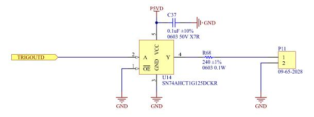
Figure 3: Trigger Out Schematic (Rev F and later)
