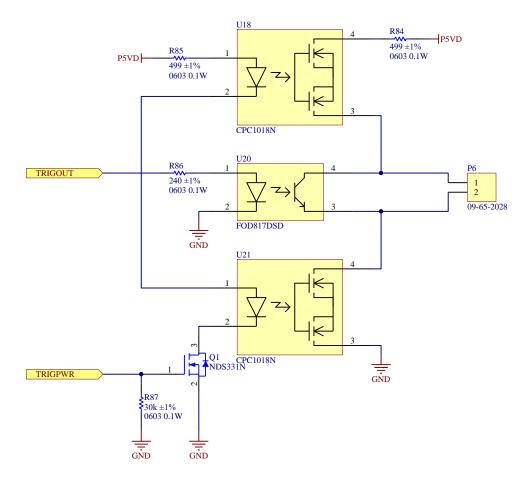
Figure 2: Trigger Out Schematic (Rev E and earlier)
