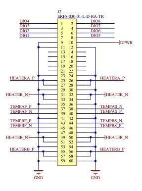
Figure 25: Heater Module Connector
