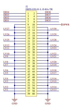
Figure 20: LVBias Module Connector
