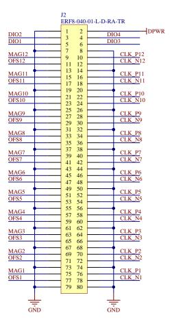
Figure 23: High Speed Module Connector
