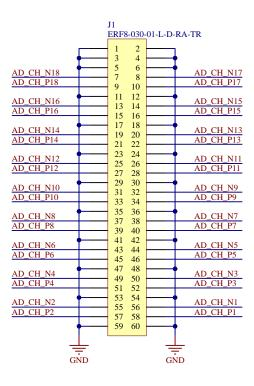
**Figure 17: ADM Module Connector**
