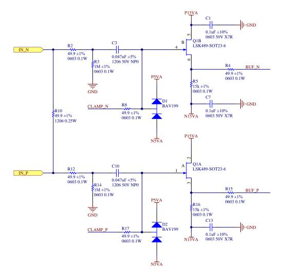
Figure 11: ADC Input Buffer
