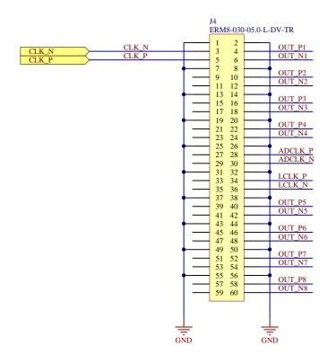
Figure 10: ADC Module Backplane Connector
