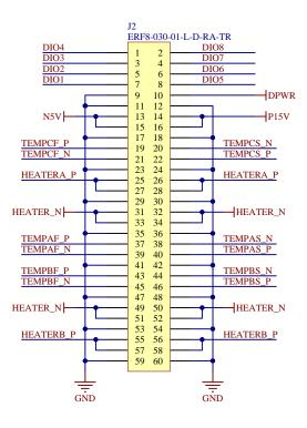
Figure 26: HeaterX Module Connector
