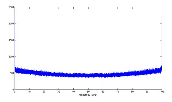
Figure 13: ADC Grounded Input FFT
