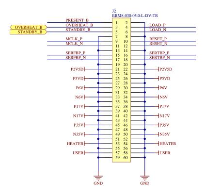
**Figure 9: Module Backplane Connector**
