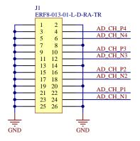
Figure 12: ADC Module Connector
