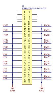
Figure 21: HVBias Module Connector
