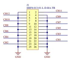
Figure 19: DriverX Module Connector
